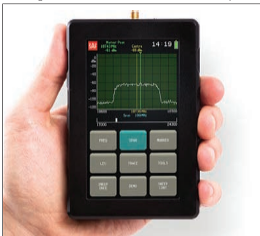
▲ Fig. 1 The Spectrum Compact is no larger than a cell phone and weighs only 10.6 oz.
